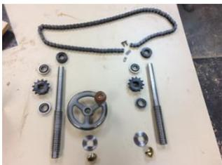
Jim is happy with the chain drive clamp. For him it was a matter of finding the right parts. The screw came from a left-over wagon vise and has left-hand threads. That allows the vise to respond with a righty-tighty, lefty-loosey clamping motion. He had a local machine shop turn down the ends to mount to sprockets and knobs for the drive systems.
