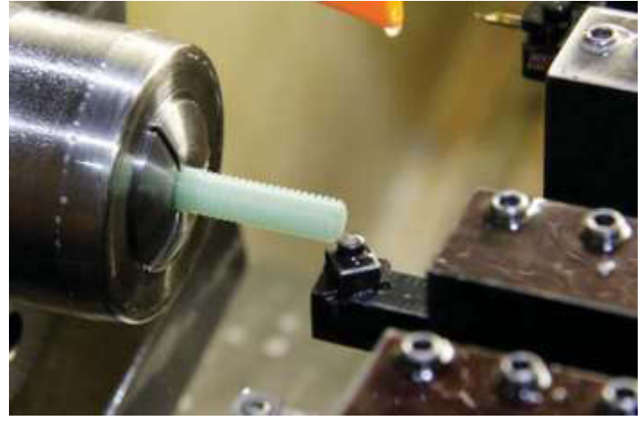
The FR4 Atlas Fibre sheet rod after machining.
