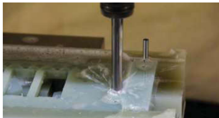
FR4 sheet being milled on a CNC milling machine.
