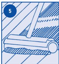
**5. STAIN:** Apply stain to the floor (if staining). Do not rub the stain in with an aggressive action. Doing so will remove Timbermate.
