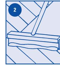
**2. APPLY:** Just before the final hard plate or screening, apply Timbermate by flooding the floor and squeegee it across the grain over the entire floor. Do not apply Timbermate too heavily – a small amount goes a long way. Remove all excess Timbermate (return excess to the Timbermate container-no waste).
