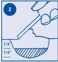
**2. FILL:** If hole is greater than 1/4", fill by layering Timbermate in 1/4" increments.
