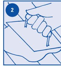
**2. APPLY:** Apply Timbermate, just before the final sand, with a plastic trowel, or rubber float across the grain over the entire floor. Make sure the filler is forced into deep voids. Do not apply Timbermate too heavily – a small amount goes a long way. Remove all excess Timbermate. (Return excess to the Timbermate container-no waste.)
