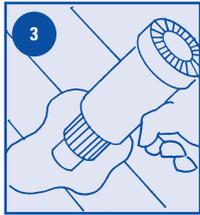
**3. DRY:** Let Timbermate dry thoroughly. Use a heat gun or similar to speed drying time if desirable. (Timbermate is properly dry if it sands to the consistency of baby powder.)
