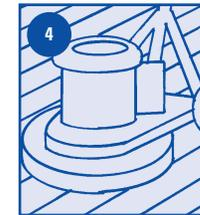
**4. SAND:** Final hard plate or screen and remove all dust and debris. (NOTE: Do not use a grit coarser than 120.)
