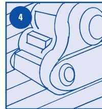
**4. SAND:** Final sand and remove all dust and debris. (If grain filling do not use a grit coarser than 120.)
